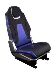
The seat system has gone from 9 to 5 links enabling industry leading foot path to the third row, increased cushion width, less weight, more streamlined design that can be easily controlled by using an app on your phone - all of this allows the seat to look just like a 1<sup>st</sup> row seat.
